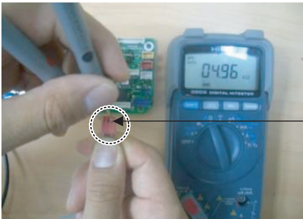
← Measure the resistance of outlet pipe temp sensor.
