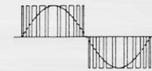
Output voltage wave-form
