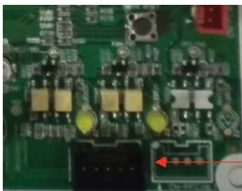
15V Input power on Inverter PCB
