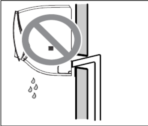
Case 1 : Indoor drain hose is high more than outdoor.
