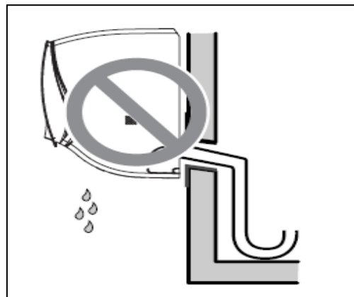
Case 6 : The end of drain hose is curled up.
