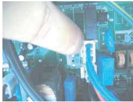
*** Indoor PCB drain pump connector (Check input of 220V) (Marked as CN-DPUMP )
