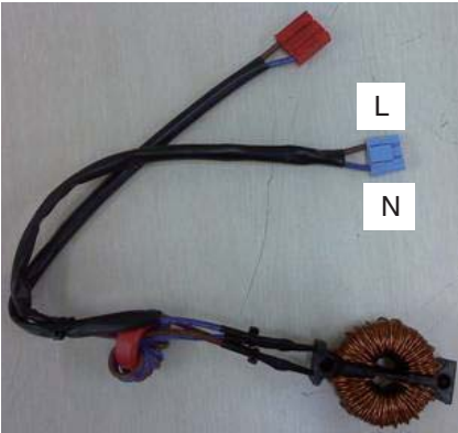
< Noise Filter wiring Check Point >
